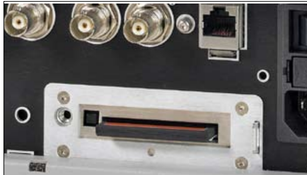
CompactFlash™ Card ejector on instrument rear side
